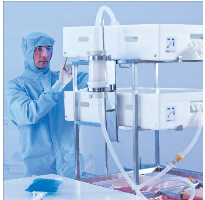
Allegro 20 L trays and trolley used in a typical filtration application
